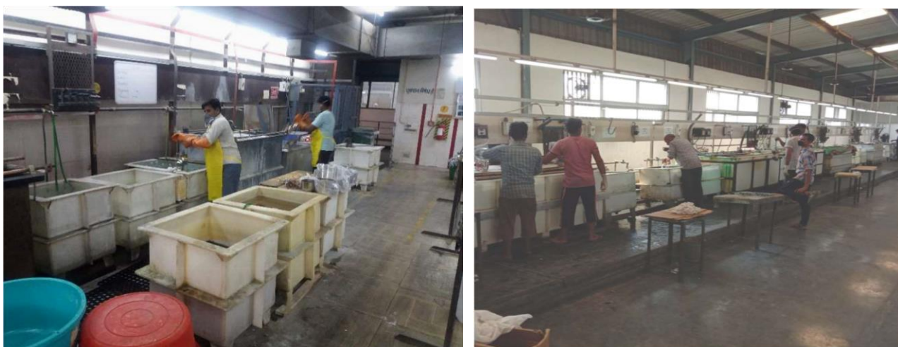
Fig. 3 Various types of Electroplating process are in electroplating unit of metalware industry (layer thickness) and after article rinse in 03 separate tanks where freshwater continuously running
