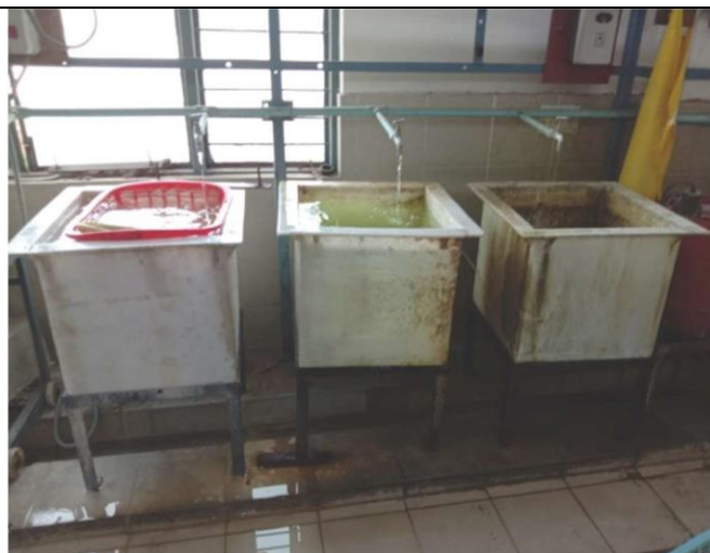
Fig. 5 Conventional rinsing - 03 separate tanks & 03 taps levels compared to the second & first tanks. Therefore, there TDS will be very minimum or we can say that it is equal to clean water but there is very unpractical system in the metal ware industries, that There continuously feed to 03 separate rinsing tanks by 03 taps during the working days of industries and after filling the tank, water is going continuously to ETP through the overflow. Which is the reason that Electroplating units of metal ware industries use a large amount of freshwater from the groundwater extraction.
